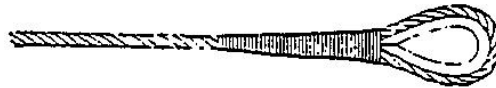
Spliced Eye and Thimble \frac{1}{2} " and smaller 100% \frac{3}{4} " to \frac{1}{2} " 95% \frac{7}{8} " to 1" 88% 1\frac{1}{4} " to 1\frac{1}{2} " 82% 1\frac{3}{4} " to 2" 75% 2\frac{1}{2} " and larger 70%
